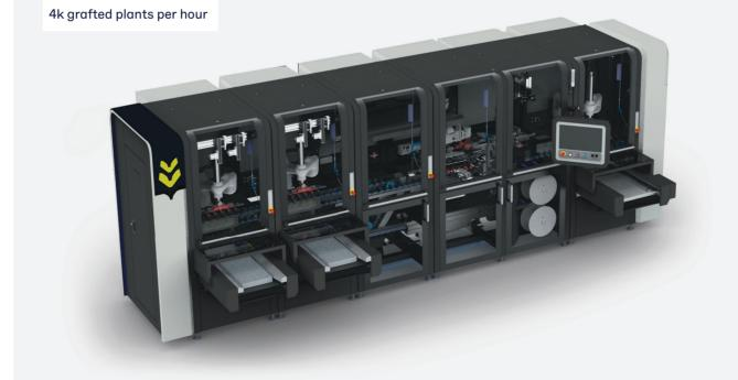
The High-Speed Grafter is the first fully automated machine for grafting both above and below the seed leaves, using vision AI and robotics to deliver up to 4,000 grafted plants per hour.
