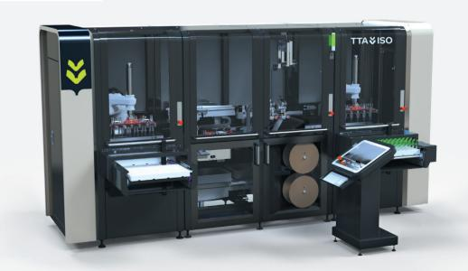
The High-Speed Clipper processes up to 4,000 clipped plants per hour, utilizing advanced vision technology and robotics to ensure reliable, high-quality results.
